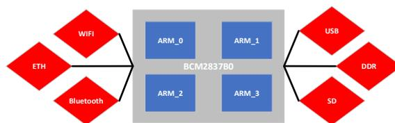
Figure 4: Architecture of the Raspberry Pi 3B+
