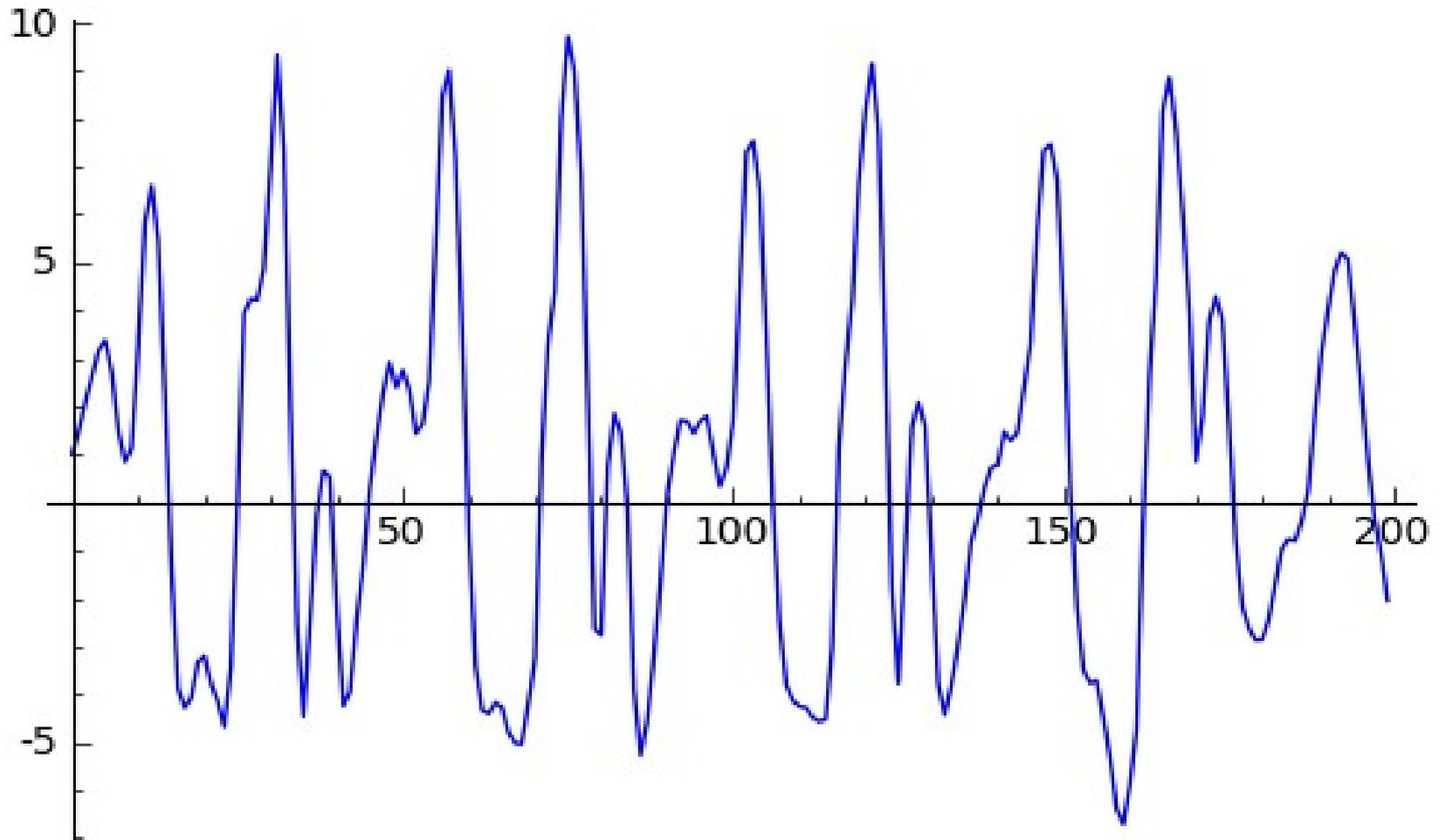
Absolute value of the a smartphone accelerometer signal when the subject was walking, device in the pocket.
